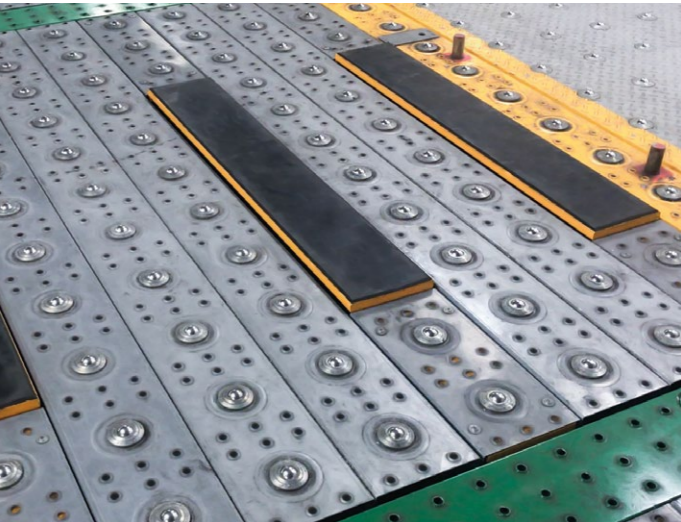
Pneumatic stops prevent the ULD from moving for safer loading processes
