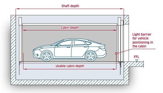
In the case of car lifts with a front- and rear-opening design, the dimensions are as follows.\*
